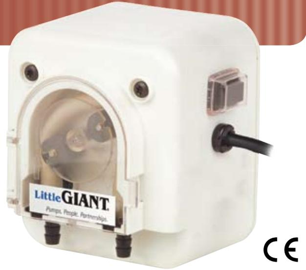
PC condensate pumps can be located in the ceiling void and lift water from wall, floor, ceiling or cassette air conditioning units up to 12 kW. Quieter than other condensate pumps, Little Giant PC pumps feature a totally enclosed motor (no ventilation required), “press-to-activate” switch, 5-minute “off” delay (PCS and PCT), easy to replace pump tube and mounting bracket.
