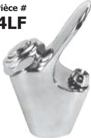
The Lyncar Drinking Fountain - Push Button features a chrome plated brass body, a Stainless Steel Cartridge and replaces HAWS HW5010. It installs onto a 3/8" Female Iron Pipe.
