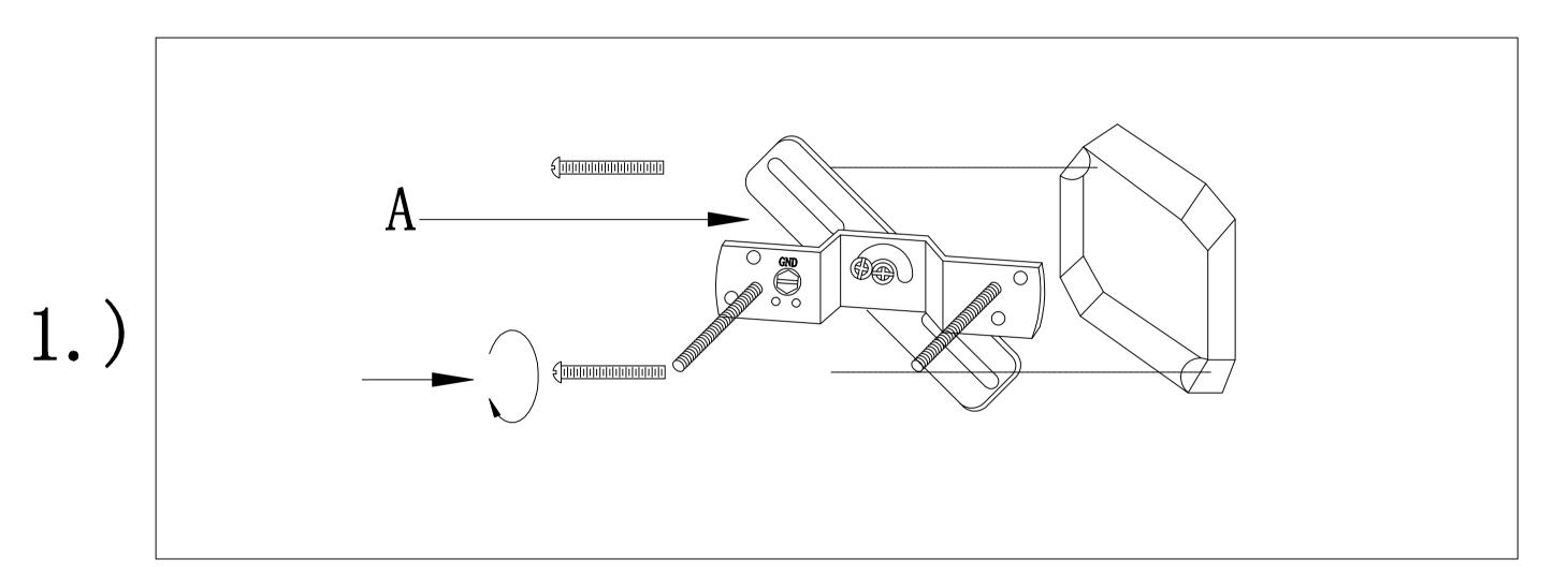
Step.1: Remove mounting bracket from fixture(B) and install to electrical box. then wire fixture to wires in outlet box. Copper wire is for Ground.
