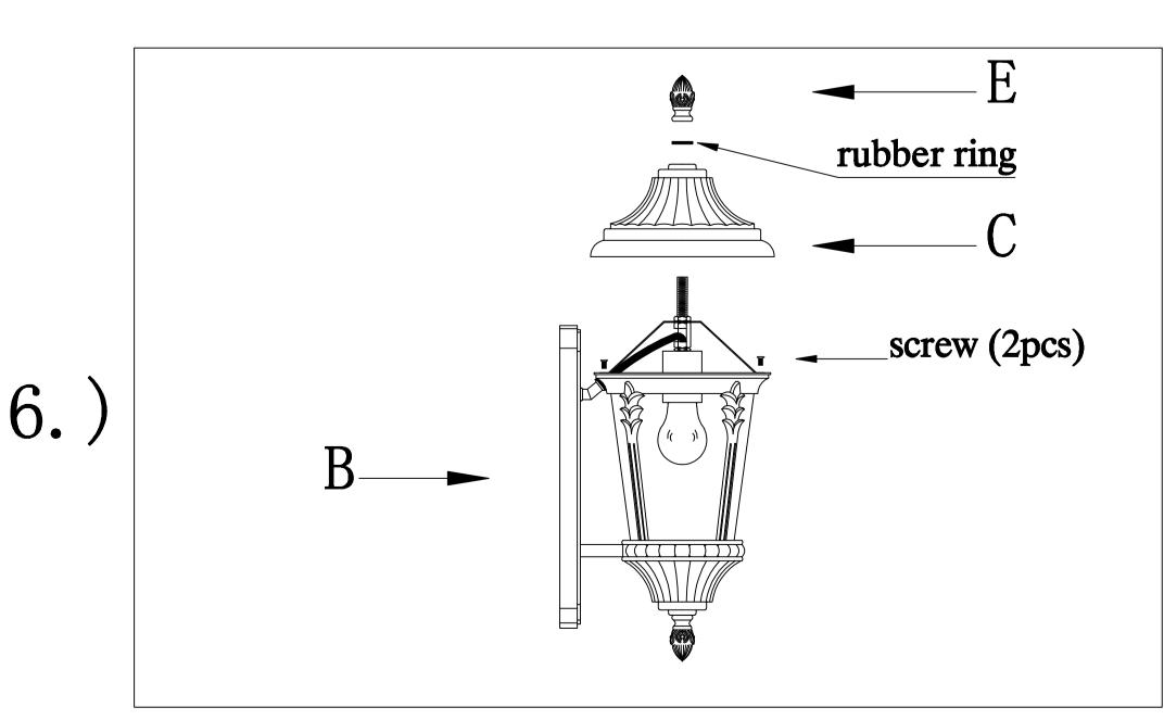
Step.6: Attach trestle to the fixture (B), using 2 screws. Attach the hood(C) and the finial(E).
