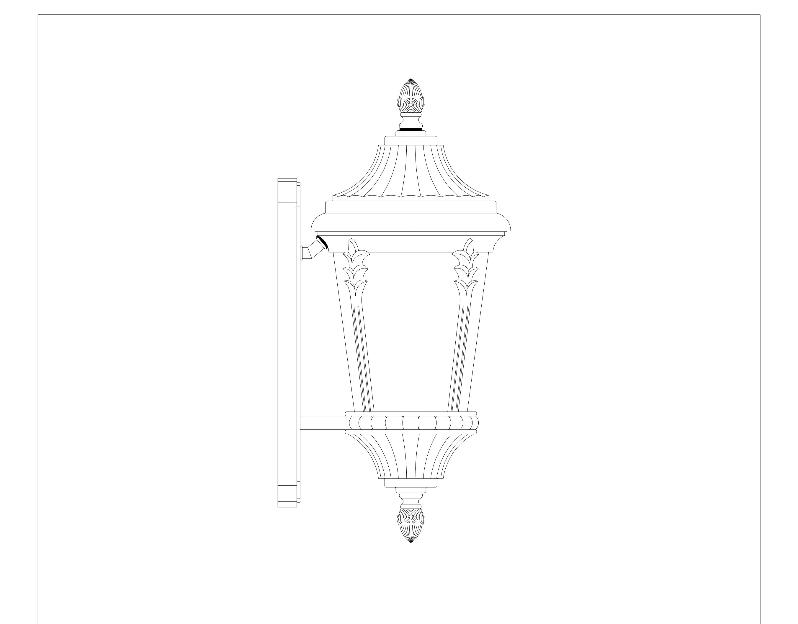
To prevent water intrusion, caulk around back-plate where fixture meets the wall using outdoor silicone sealant. Leave a small gap at the bottom to allow moisture to exit.
