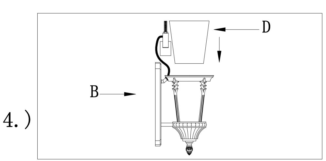
Step.4:Install the glass shade(D) into the fixture(B).
