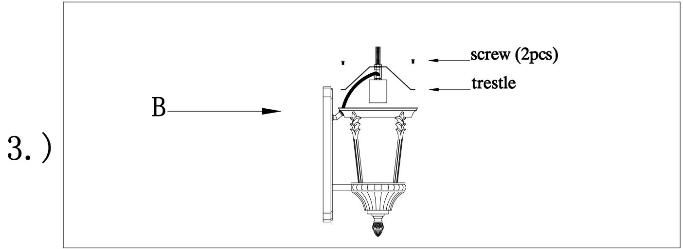
Step.3: Remove 2 screws and loosen the trestle.
