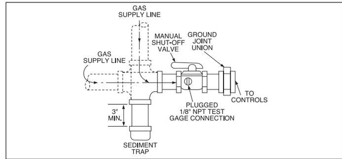
① Manual shut-off valve is in the "OFF" position when handle is perpendicular to pipe.
