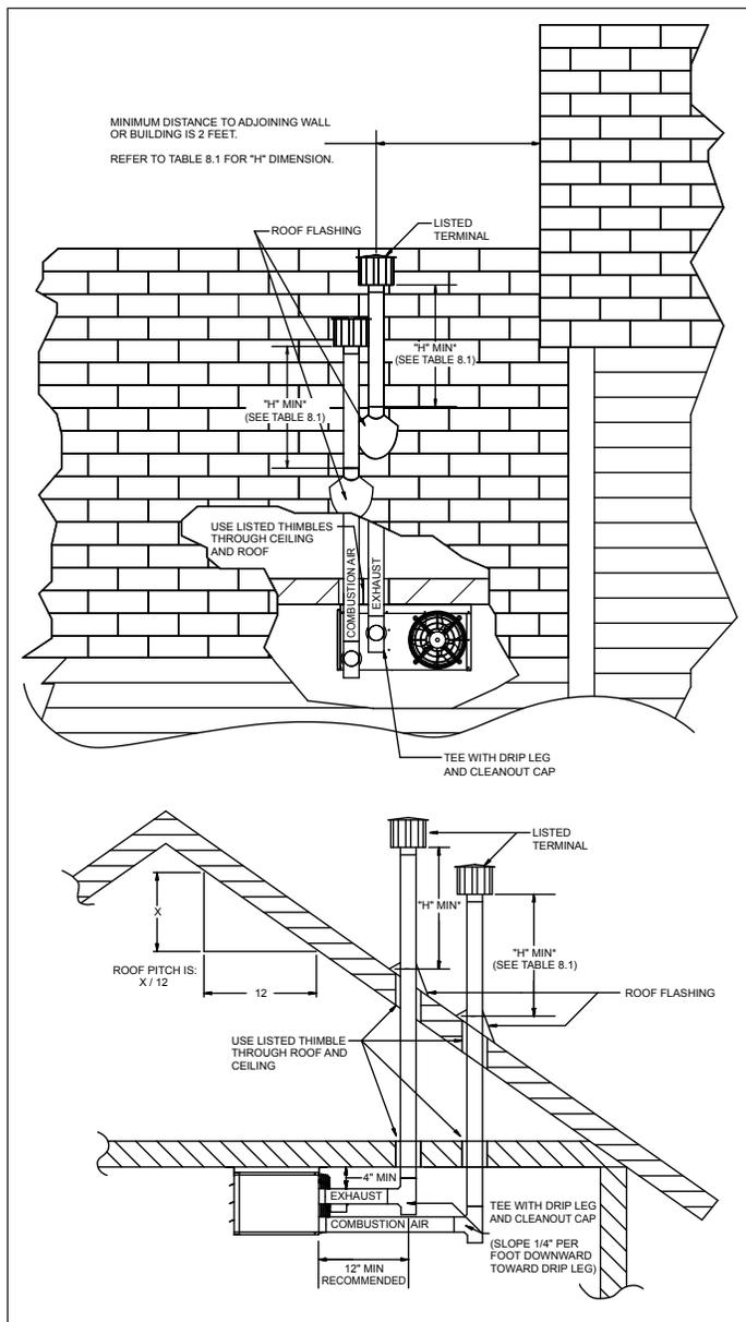
**Figure 8.2 - Vertical 2-Pipe Vent System - Flat Roof**
