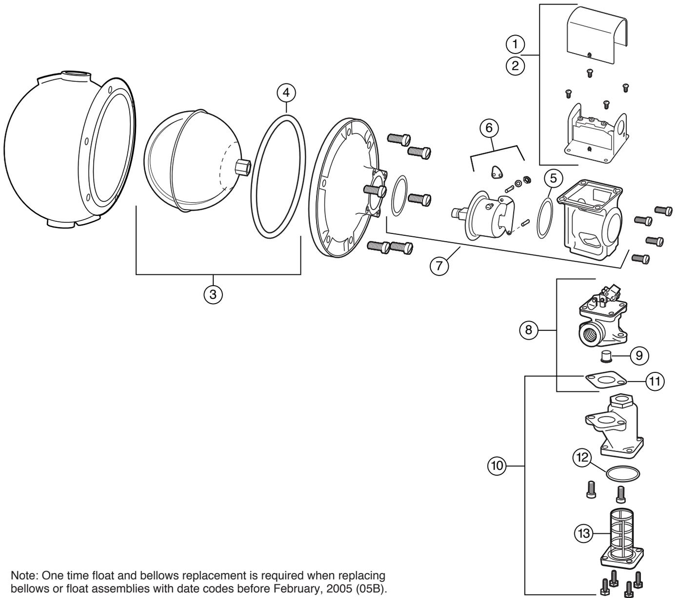
Note: One time float and bellows replacement is required when replacing bellows or float assemblies with date codes before February, 2005 (05B).
