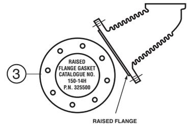
This new gasket, specifically designed for the Raised Flange Heads, may be used.
