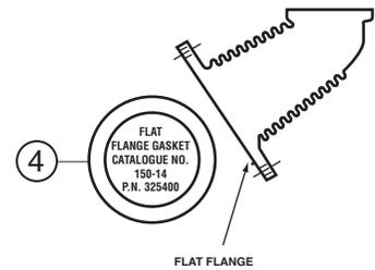
This gasket **must** be used on the Flat Flange Heads.
