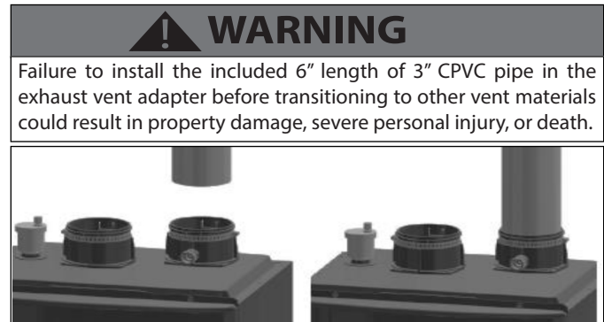
Figure 19 - Correct Installation into the Boiler Collar
