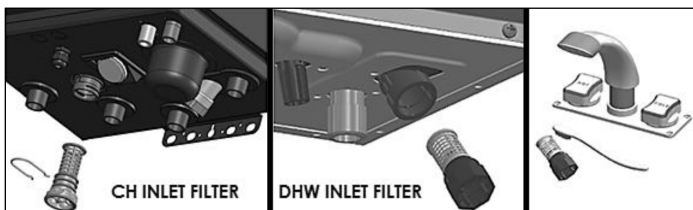
Figure 58 - Cleaning the Inlet Filters
