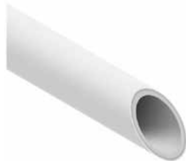
CoolPro pipe is extruded with an outer layer containing 30 year UV-Resistant white PPR material.
