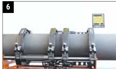
6 Final Welding / Cooling
