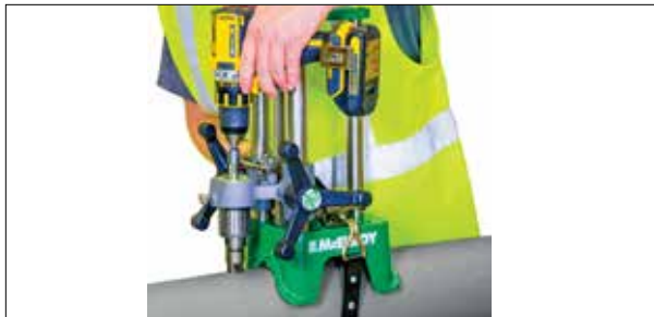
A McElroy hornet tool is pictured here clamped onto the pipe and into position.
