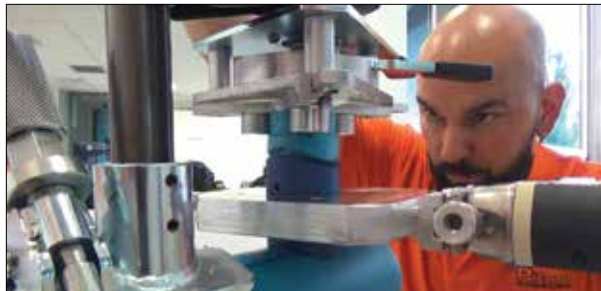
A machine-assist tool allows the branch to be aligned perpendicular to the main. Pictured here is a Ritmo Up 125 Machine.
