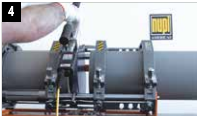
4 Bead-up (Initial Welding)
