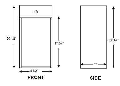
National Fire's Classic series are surface mounted cabinets that are both practical and economical. Theft and vandal resistant; these cabinets remain locked at all times, allowing emergency access through means of breaking the scored plexi glass. Cabinets come complete with scored plexi, breaker bar, key and decal. Perfect for parking garages, warehouses, industrial areas and construction sites.
