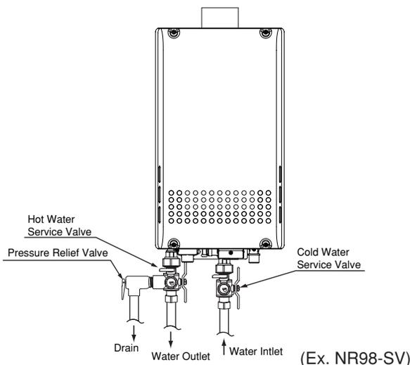
\* Isolation valves may be purchased as an accessory from Noritz. They allow for full diagnostic testing and easy flushing of the system.
