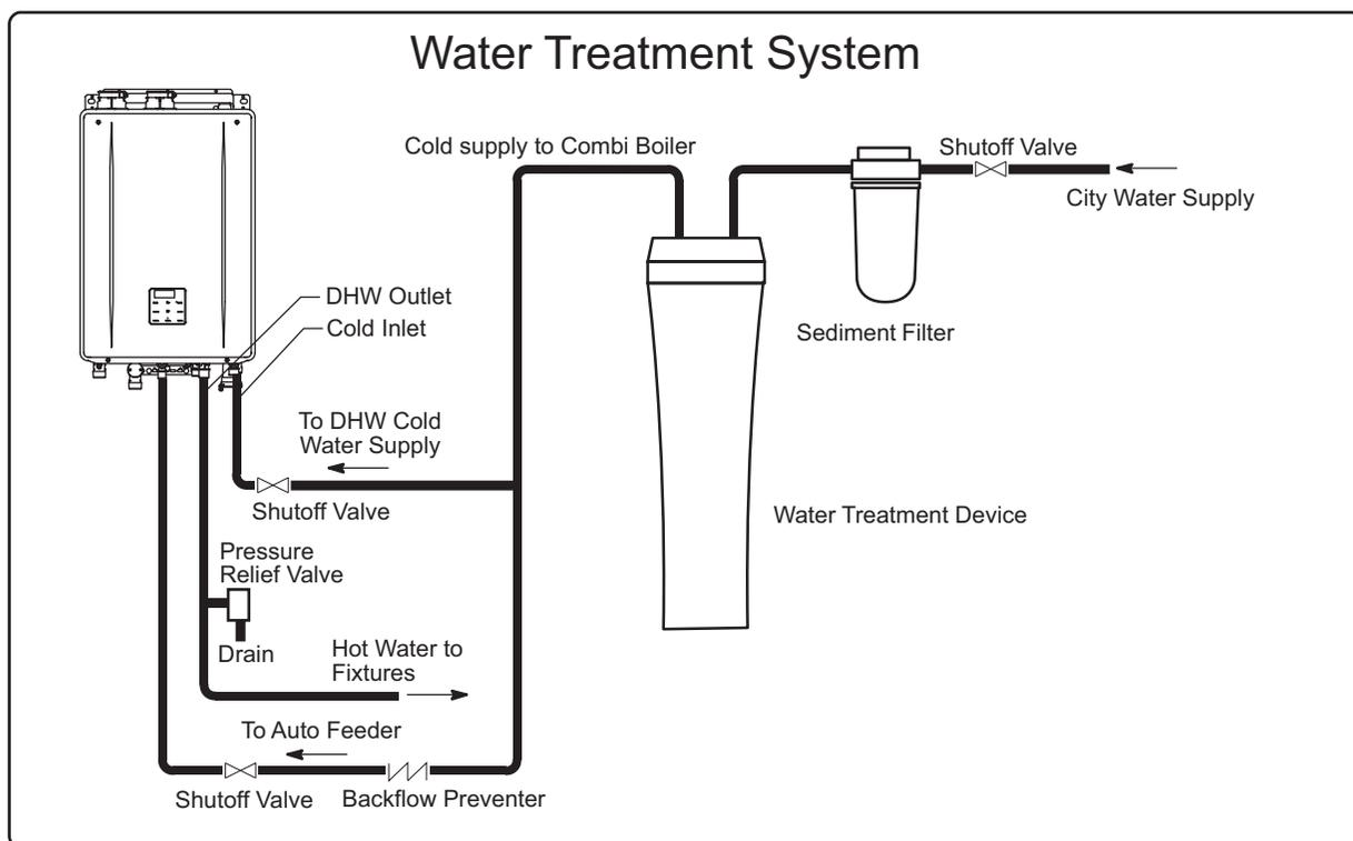
▲ The illustration is an example. Please check with the actual Combi Boiler about the position of piping, and form.
