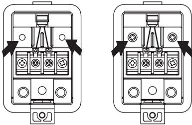
4. There is a through hole to pass wire into the case.
