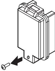
2. Remove the cover by lifting it and pulling it outward.
