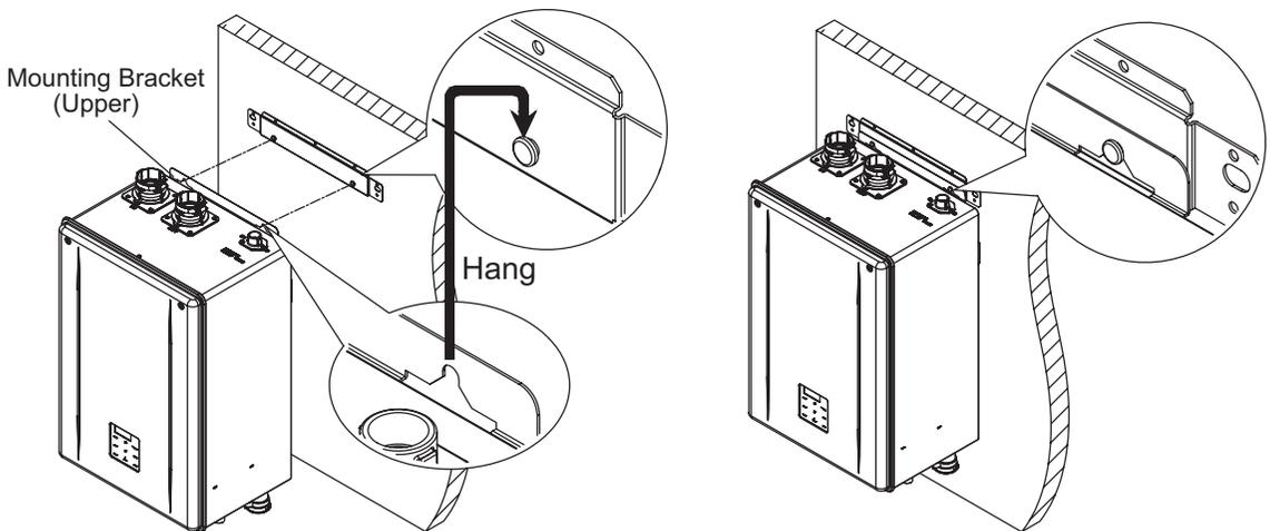
2. Hang the Combi Boiler on the Wall Mounting Bracket.
