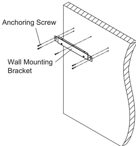
1. Drill holes for the Wall Mounting Bracket. Affix the Wall Mounting Bracket securely to the wall by 5 screws. Ensure that it is leveled, and it can support the weight of the Combi Boiler.
