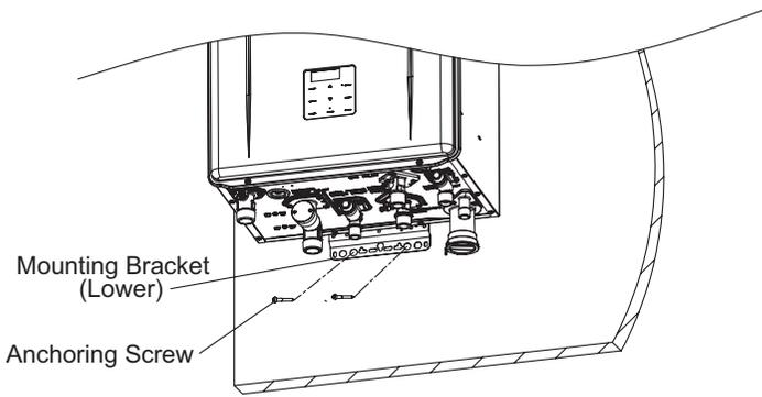
3. Affix the Mounting Bracket (Lower) to the wall by 2 screws.
