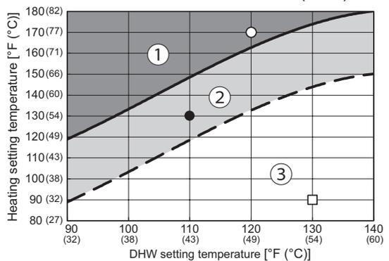
\* The "3" area is unavailable for simultaneous operation.
