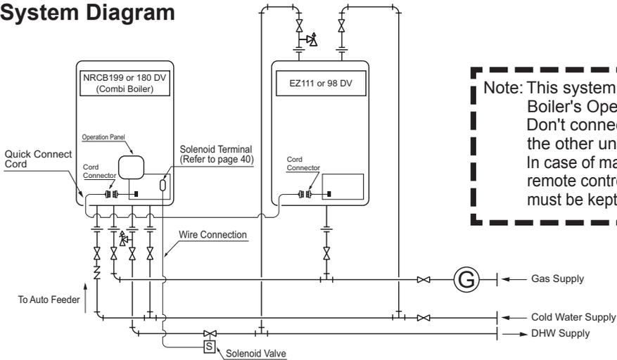
Note: This system is operated by the Combi Boiler's Operation Panel. Don't connect the remote controller to the other unit. In case of maintenance, EZ111 or 98 DV's remote controller (Included Accessory) must be kept by the customer.
