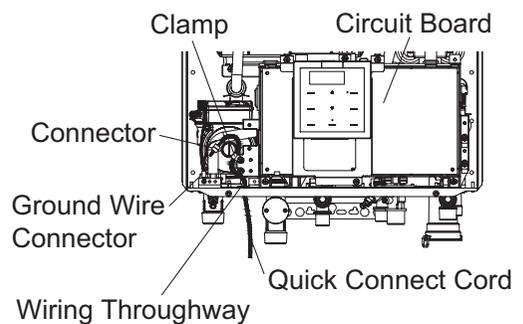
\* Connecting the cord to the other unit, refer to the unit's Installation Manual.
