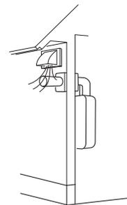
State of California: The Combi Boiler must be braced, anchored or strapped to avoid moving during an earthquake. Contact local utilities for code requirements in your area or call: 1-866-766-7489 and request instructions.
