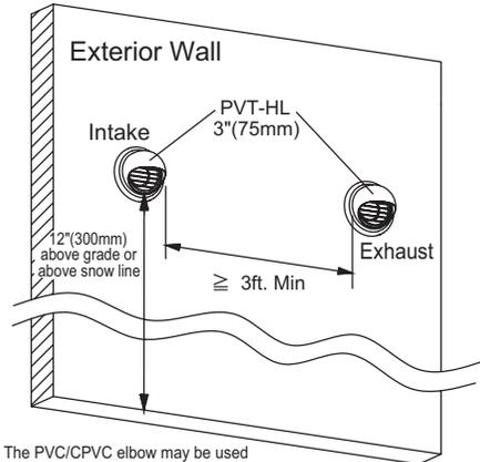
When choosing intake and exhaust terminations, you must use the same type of elbow (i.e. both 90° elbows). This will help with proper combustion by putting both terminations in the same pressure zone.
