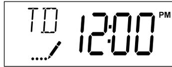
Adjust the displayed time with or buttons. Press to resume normal operation
