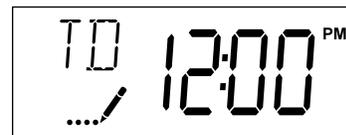
12. Set time of the day in the control valve and program the user section of the control. Refer to control valve programming section in this manual.
