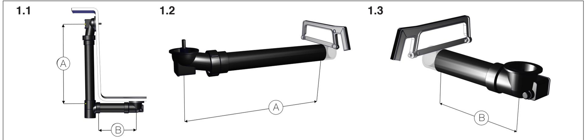
1.1: When measuring, dry fit tubing approximately 1" (2.5cm) into Tee, overflow Ell and drain Ell. Cut accordingly.
