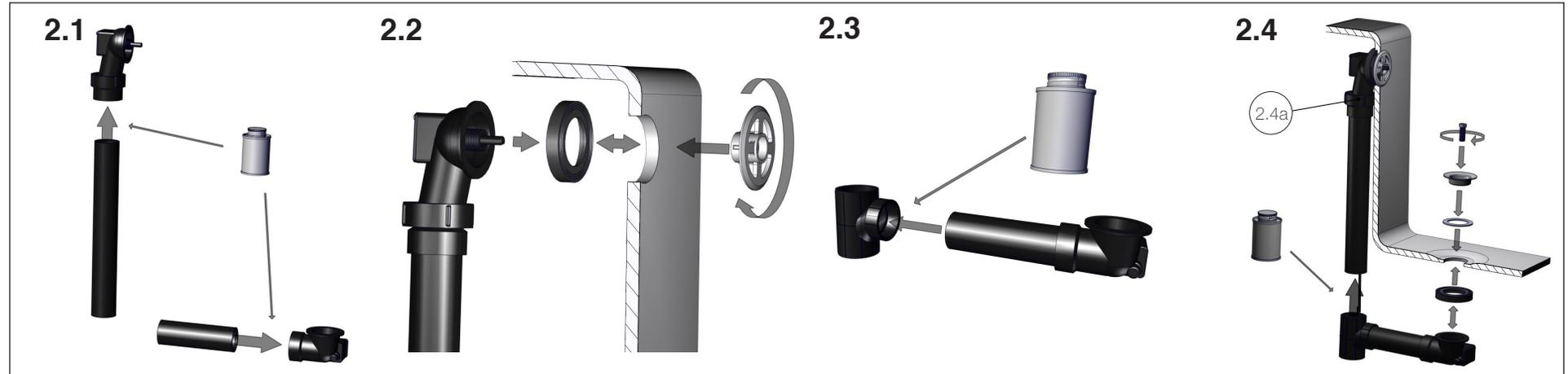
2.4a: After gluing all joints\*, hand tighten Nut until snug.
