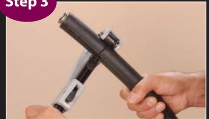
Using the appropriate tubing cutter with TracPipe #FGP-E-5272 Cutting Wheel, score the black sleeve approximately half of the way through. Use extreme care not to cut down to the stainless corrugated pipe. No more than two turns in on the cutter is sufficient. Inspect tube for scoring from the tubing cutter.
