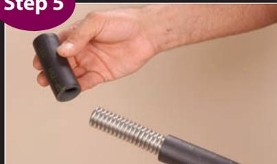
Using a twisting motion, remove the black sleeve and yellow jacket from the pipe. It may be necessary to cut sleeve longitudinally and peel off on larger sizes. Inspect stainless pipe for scoring from the tubing cutter.
