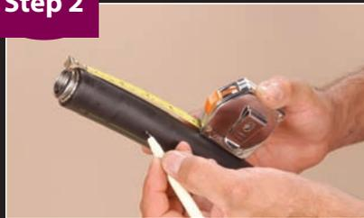
Mark the sleeve at specified length on the Strip Length Chart (above) – plus 2".
