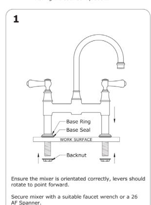
Ensure all connections are firmly tightened
