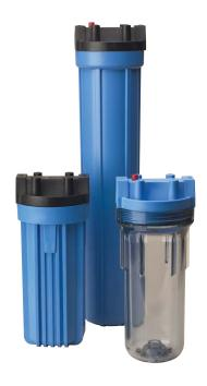
Pentair Standard Filter Housings are manufactured of a durable polypropylene or clear Styrene-Acrylonitrile (SAN). All are equipped with 3/4" NPT inlet and outlet ports. Standard Filter Housings are available in both 10" and 20" lengths and will accommodate a wide range of 2-1/2" to 2-7/8" diameter cartridges. The reinforced polypropylene cap offers an optional pressure-relief button on the inlet side to relieve pressure inside the housing when changing filter cartridges.
