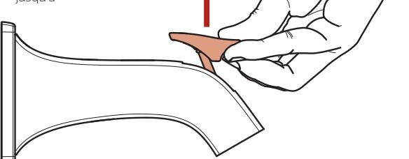
To return the diverter to its normal position, shut the water off and let it drain. If necessary, push down on the diverter after the water has been drained.
