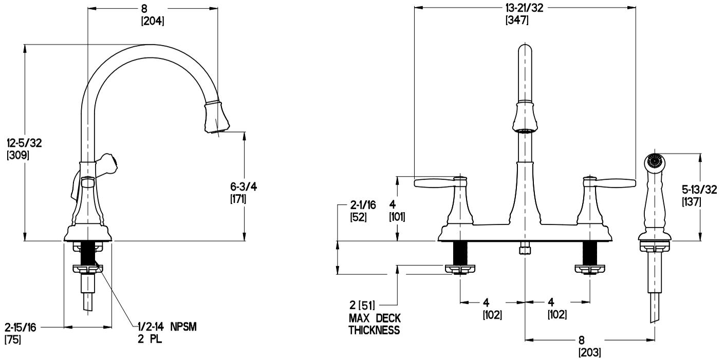
Ø1-3/8 Min to Ø1-1/2 Max. Deck Hole Openings
