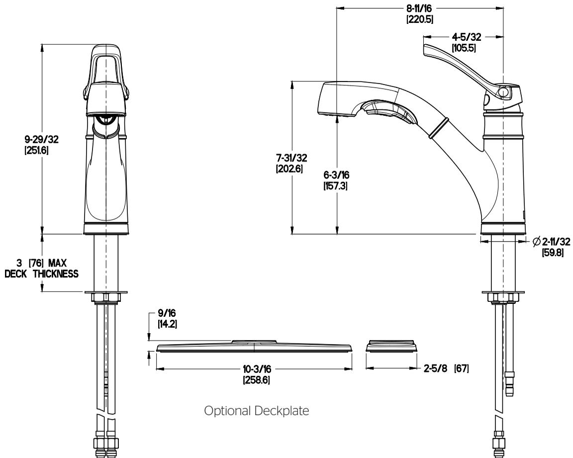
Ø1-3/8 Min to Ø1-1/2 Max. Deck Hole Openings
