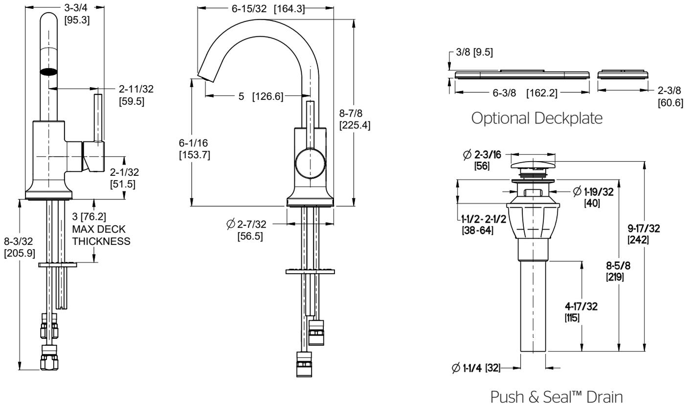
Ø1 Min to Ø1-1/2 Max. Deck Hole Openings
