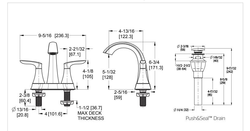
Ø1 Min to Ø1-1/2 Max. Deck Hole Openings
