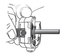
3. Rotate until the pipe is cut.
