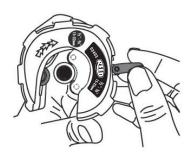
1. Flip handle up and rotate handle to adjust the slide block to the desired size mark.
