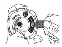
2. Insert pipe into the cutter and rotate as indicated by the arrows on the side of the body.
