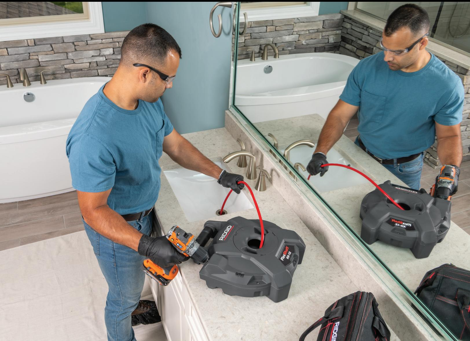
The NEW RIDGID® FlexShaft K9-12 machine is the most compact version of the FlexShaft Drain Cleaning Machines. The fully enclosed housing contains 30' of FlexShaft cable, encapsulated in nylon sheath for less mess and easy cleanup. The lightweight, portable design is perfect for 1¼" - 2" pipes.
