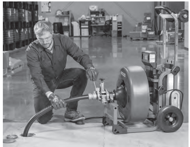
Figure 23 – Using Machine with Guide Hose
