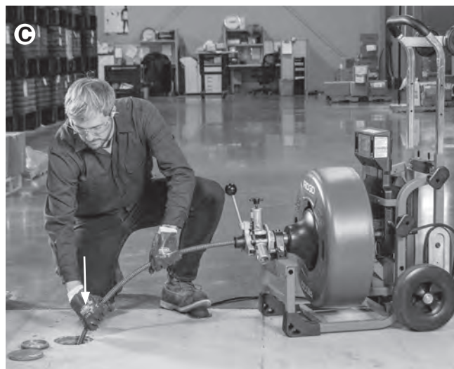
Figure 20A,B,C – Manual Feed Operation
