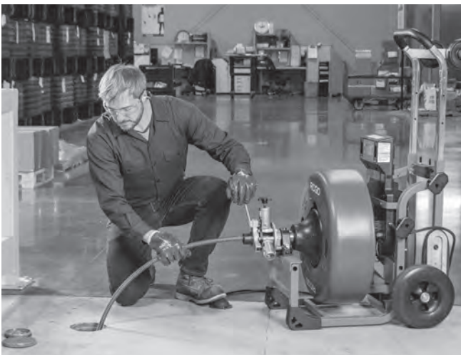
Figure 21 – Operating using the AUTOFEED Unit
