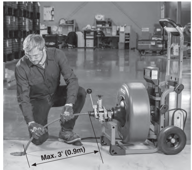
Figure 17 – Proper Operating Position
