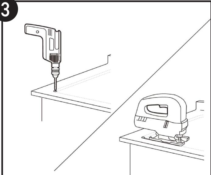
Drill a pilot hole and cut the countertop opening. Use the appropriate cutting tool for the surface you are cutting and cut along the inside of the template line.
