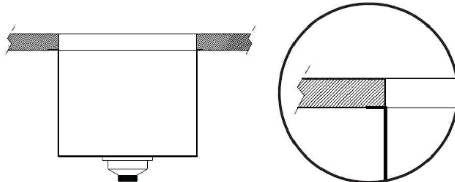
These instructions are for installing ROHL Undermount stainless steel sinks. By Undermount, one identifies a sink that is installed from below the countertop.
