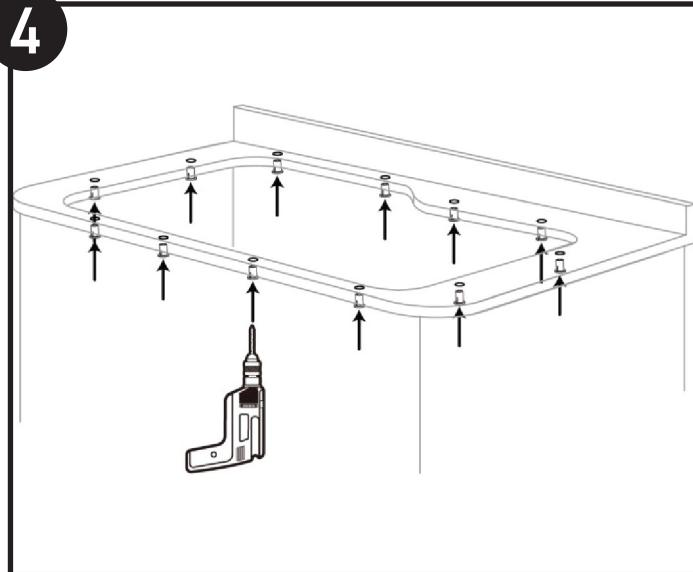
On the underside of the counter, mark the location of the twelve holes for the clips. These holes should be equally spaced around the perimeter of the cutout. Using an electric drill with a 11mm drill bit, drill each hole so that it is 11mm in diameter and 14mm deep. Insert the plastic caps from each of the clips into each of the installation holes.
