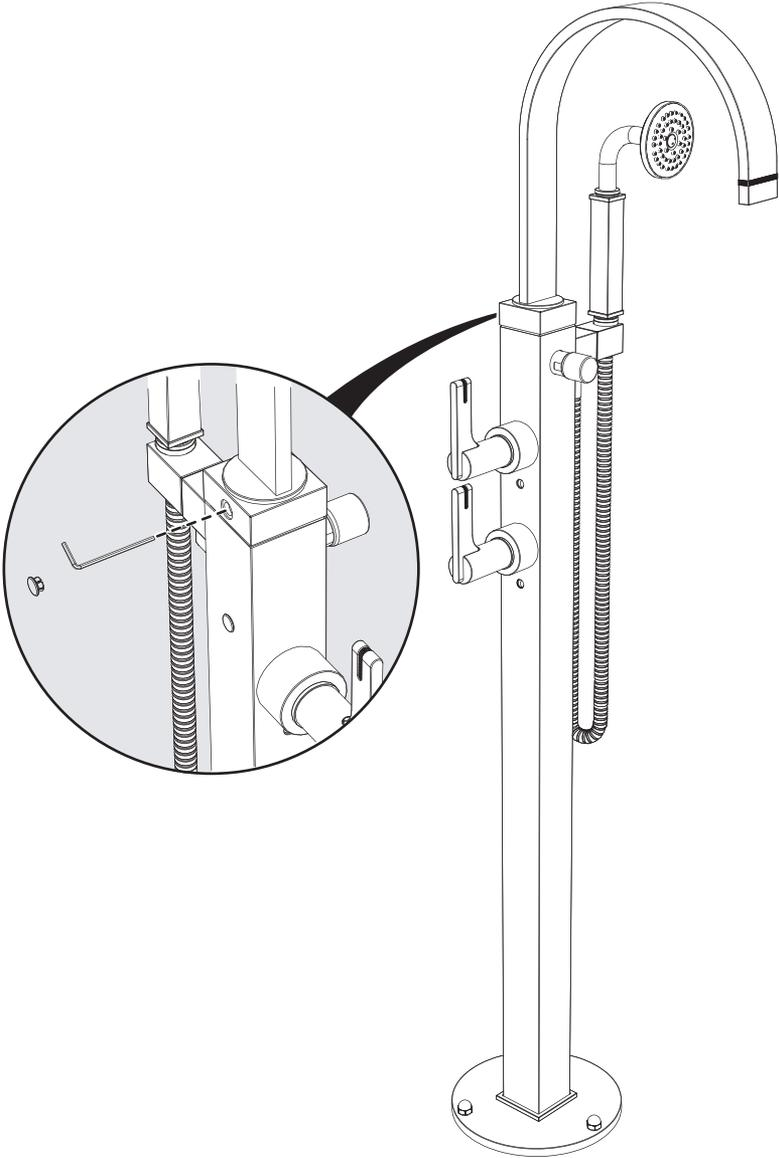
\* Place the index cap after tightening the set screw.
