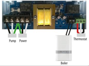
Make sure that the fuse is 5A, slow blow and inserted correctly.
