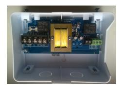
Disconnect the AC power to the AC wiring for the device.
