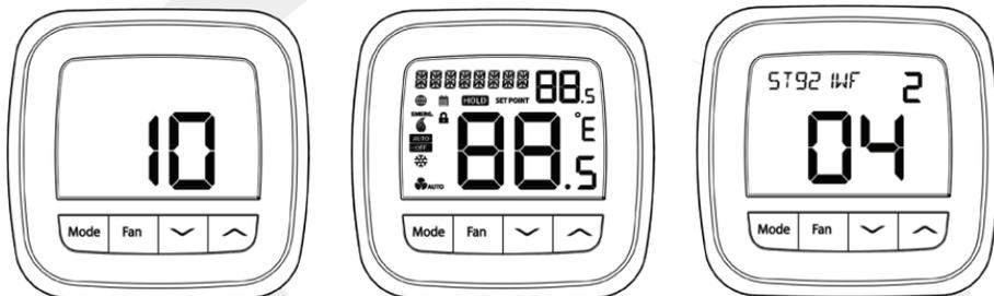
When the ST921WF is first powered or if a Factory Reset is performed, the above boot sequence will be displayed. The last screen displays the thermostat model and firmware version number.
