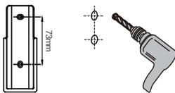
Drill two holes with a diameter of 4.5mm in the wall according to the position of holes on the remote control holder
