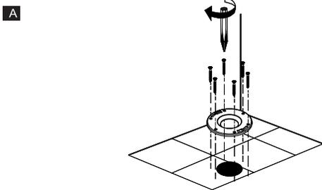
Install the floor drain cover connector(not included) .
