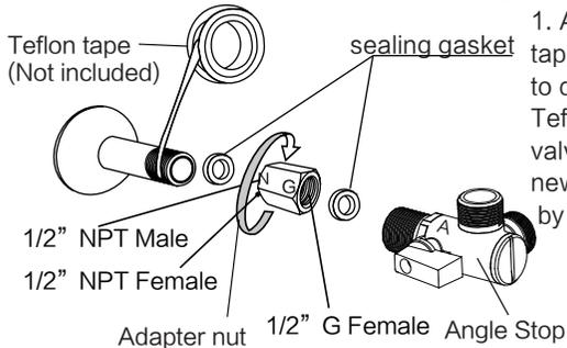
1. After external thread of water outlet hose is wrapped with Teflon tape, adapter nut need install sealing gasket, tighten the adapter nut to direction N, then after external thread of angle stop is wrapped with Teflon tape, and tighten the connecting nut to direction G. If the angle valve has been installed on the wall, to ensure proper installation of new angle stop, the angle valve shall be replaced with the angle stop by professional personnel.
