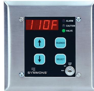
System to include key access programmable electronic module, stainless steel panel, 4" x 4" electrical mounting box, 120V AC - 12V AC/15VA UL Listed/CSA Certified Class 2 transformer, solid state temperature probe with 25' of cable and (2) system operation keys.
