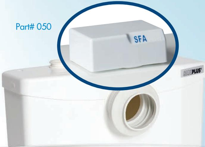
The Sanialarm has a level pressure switch that triggers an alarm fixed on the top of the unit if the volume of water exceeds the maximum allowed level. The alarm emits a continuous 80 dB warning sound until it is switched off or the problem is rectified. The Sanialarm is battery operated and can be installed on most Saniflo macerating units and drain water pumps.
