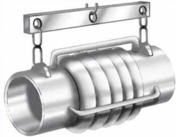
1. The opening into which the expansion joint will be installed should be examined to verify that the opening for which the expansion joint was designed does not exceed the installation tolerances designated by the designer and/or purchaser. If the opening exceeds the tolerance, notify Senior flexonics at once for a disposition.
