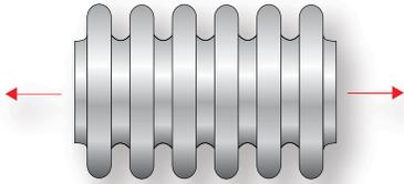
**Axial Extension:** Increase of the bellows length due to pipe contraction.
