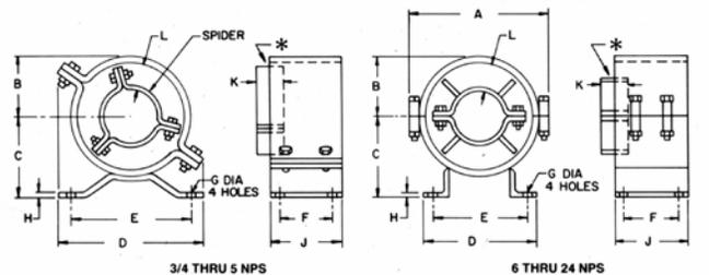
\* For maximum movement, install spider with half its length extended.
