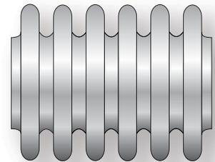
Flexibility of the bellows is achieved through bending of the convolution sidewalls, as well as flexing within their crest and root radii. In most cases, multiple convolutions are required to provide sufficient flexibility to accommodate the expected expansion and contraction of the piping system.
