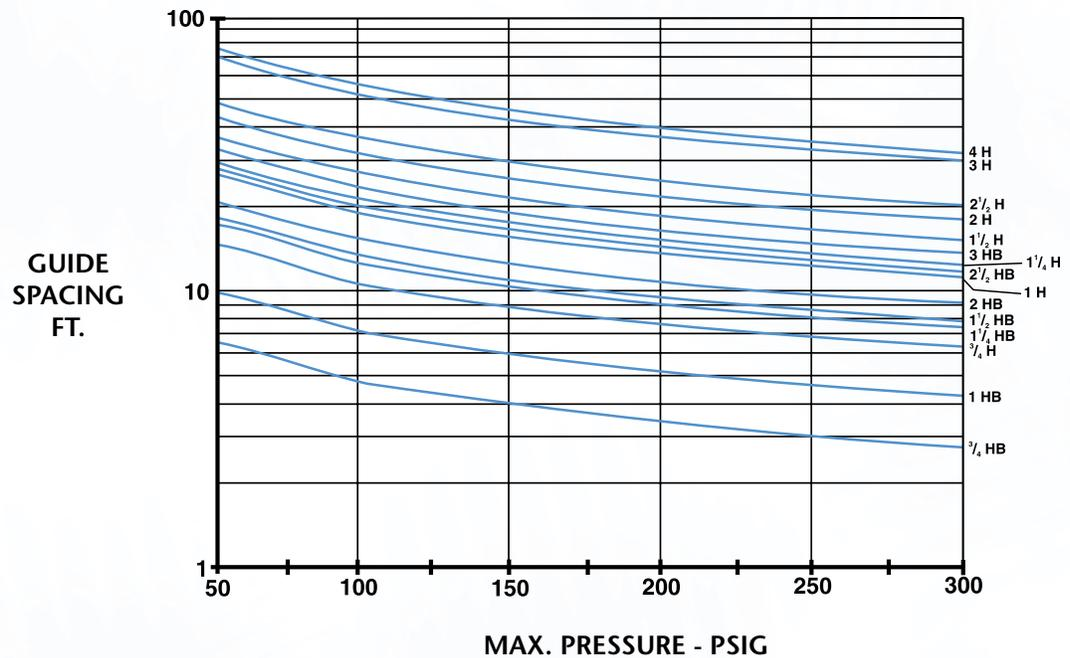
Chart is based upon sch. 40 pipe and type K copper tubing.
