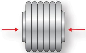
**Axial Compression:** Reduction of the bellows length due to piping expansion.
