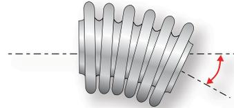
**Angular Rotation:** Bending about the longitudinal centerline of the expansion joint.
