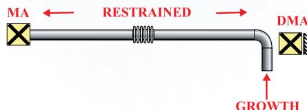
Directional main anchors are, as the name implies, intended to anchor the piping system in one direction, while allowing movement to occur from a transverse direction.
