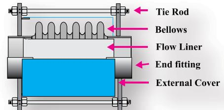
Expansion joints that are installed within ten pipe diameters downstream of elbows, tees, valves or cyclonic devices should be considered to be subject to flow turbulence. The actual flow velocity should be multiplied by 4 to determine if a liner is required per the above guidelines. Actual or factored flow velocities should always be included with design data, particularly flow that exceeds 100 ft./sec. which require heavy gauge liners.
