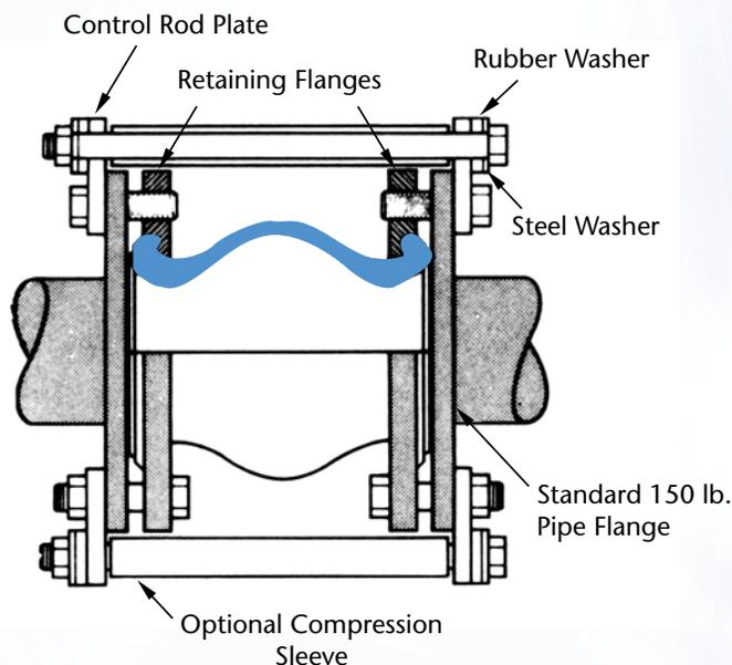
Typical example of a tie rod arrangement. Depending upon size/pressure, two or more rods will be required.
