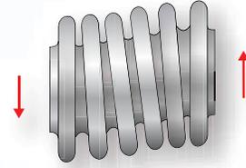
**Lateral Offset:** Transverse motion which is perpendicular to the plane of the pipe with the expansion joint ends remaining parallel.
