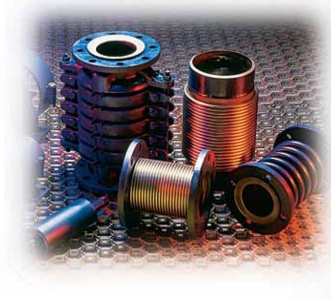
**Exhaust Flexible** Connectors (shown on page 27) are designed for low pressure applications such as stationary and marine gas turbine, diesel engine exhaust, and low pressure ducting. Large motion capability, low spring forces and reduced weight make this product ideally suited for thin-wall duct systems.
