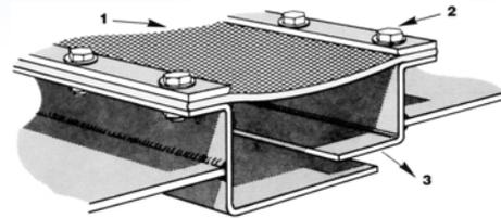
Expansion joints are offered in either integral flange or belt-type geometry. They are designed not only for relieving stress due to thermal conditions but to eliminate transmission of vibration caused by fans and other equipment in ducting systems.
