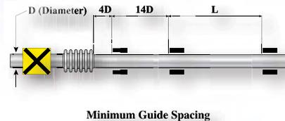
The first pipe guide must be located within four pipe diameters of each side of the expansion joint and a second guide placed within 10-14 pipe diameters of the first guide. Additional guides may be required based on guide spacing tables that consider diameter and system pressure. A convenient intermediate guide spacing chart is provided on page 23.
