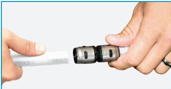
**STEP 2** Push the pipe into the fitting firmly (a twisting action reduces insertion force). Take care to avoid inserting the pipe at an angle.
