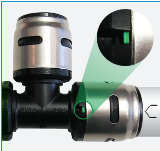
**STEP 3** Ensure that the pipe is pushed into the fitting fully and engaged properly by checking that the green indicator ring is fully visible in all four slots. This ensures a permanent connection.
