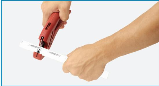
**STEP 1** When cutting SharkBite PEX Pipe, ensure that the ends are cut square and the surface is smooth. Ensure that both the EvoPEX pipe and fitting are clean and free of dirt and debris in preparation for making a connection.
