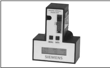
The Ammeter Display Units plug into the Sensitrip Trip Unit and displays the phase current flowing in the breaker. They are powered by the breaker's CT's with replaceable battery back-up for maintaining trip and max logs.
