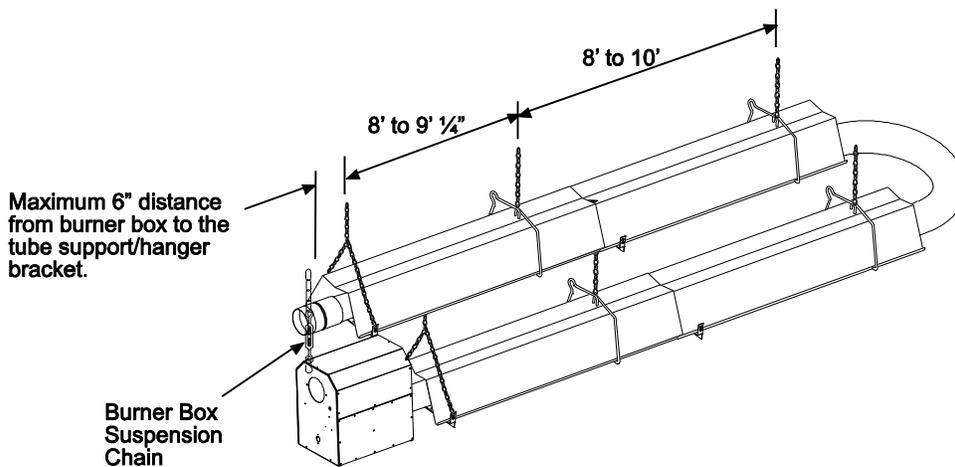
**6 hanging points to be used for suspension for a typical 40ft long system. There must be two hanging points on the first tube and one on each of the other tubes**
