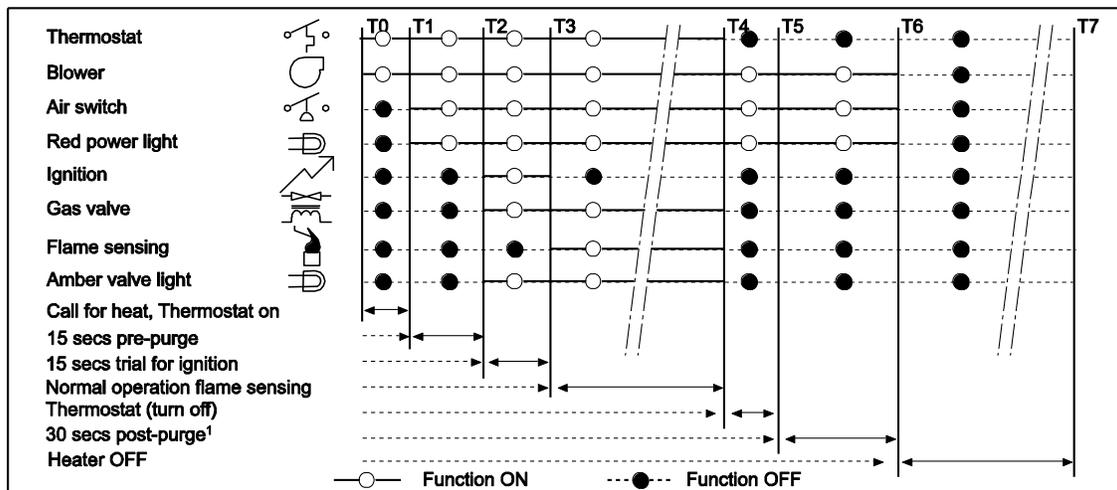
Note: When the SPS / SPU is operated by a thermostat interrupting the line voltage (120V) to the heater then the post purge function is disabled.
