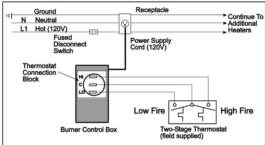
**B. LOW VOLTAGE (24V) THERMOSTAT CONNECTIONS – MULTIPLE HEATERS**
