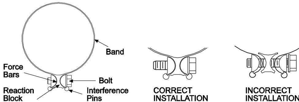
8. Check to ensure that the hardware is completely closed and the band is seated on the reaction block and interference pins as illustrated above.
