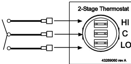
Use these three terminals for the 24V thermostat connection.
