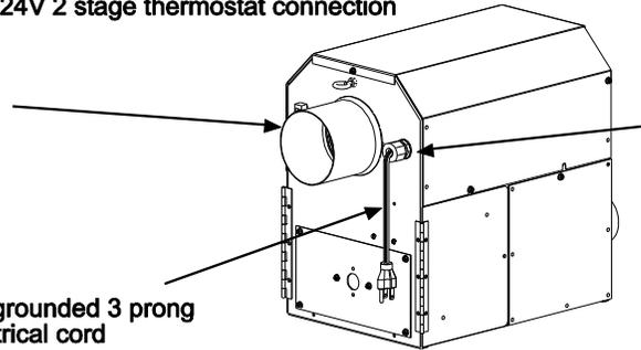
Liquid tight fitting must be tight to prevent ingress of moisture
