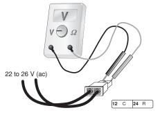
Test the Powered Inputs -
