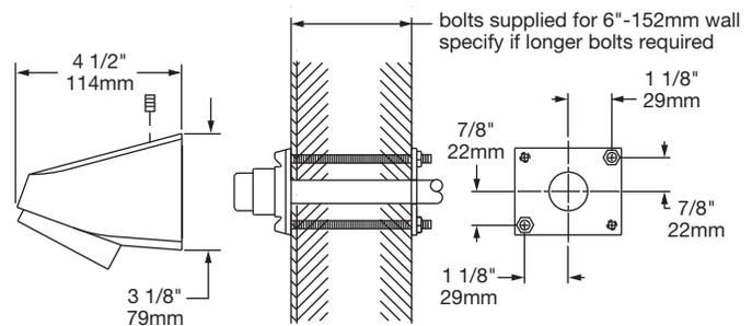
Anchor plate used for ceramic tile application—plate screws to wall and tile is applied up to sides of plate. Mounting bracket is mounted on finished wall with machine screws into anchor plate.
