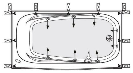
Finish the wall as shown in the image below. Apply additional silicone to seal any gaps in the corners. Clean off excess silicone on the surface of the tub immediately with a cloth and warm water.
