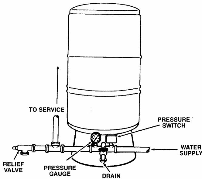
The water system tank should be installed as close as possible to the pressure switch (24 inches or less) to reduce the adverse effect of friction loss and elevation differences.
