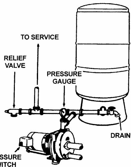
4. If your system is capable of exceeding a working pressure of 100 psig (typically submersible pumps), install a pressure relief valve (rated at 100 psig or less, but greater than turn off pressure) in the system near the tank. The valve should be the same pipe size as the tank outlet. This is not necessary on tank-mounted jet pump units.
