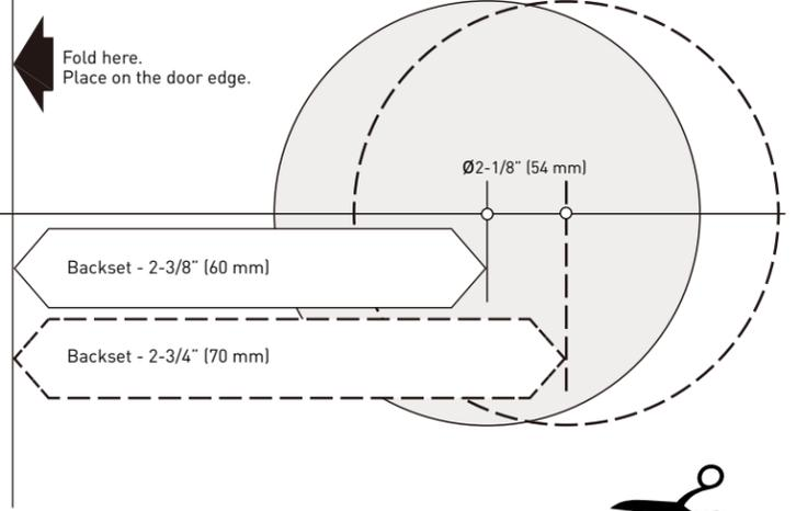
**NOTE:** For beveled doors, apply template to pull side of door.
