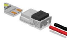
**3.** Insert light engine and wires accordingly from two sides of the connector. Do not strip ends of wires prior to insertion. Only use 20 AWG wire.
