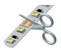
**1.** Locate un-soldered cut-point and cut UNITI light engine to the required length.
