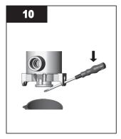
Pry sleeve upwards using sleeve removal tool until it comes loose.
