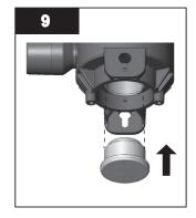
• Insert the sleeve removal tool at the bottom of the sleeve.
