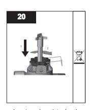
• Insert new lamp into chamber and lock into place using a quarter turn clockwise.
