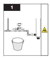
Shut off the water line to chamber and release system pressure before servicing.
