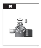
Reinstall the new lubricated orings over the top end of the sleeve.
