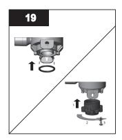
• Reinstall the O-ring at the bottom of the sleeve.
