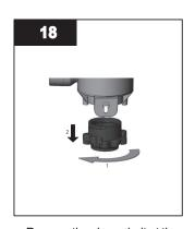
Remove the sleeve bolt at the bottom of the sleeve assembly.
