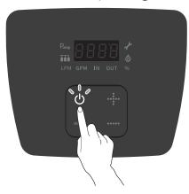
When the water heater is on, the water temperature which has been set recently will appear on the digital display.
