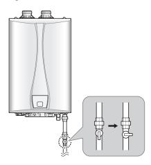
4 Turn off the water supply valve on the inlet to the water heater.
