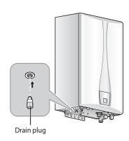
**8** Close the drain valve when the water is completely drained.
