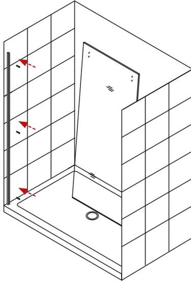
3.2 - Install the wall profile into place.
