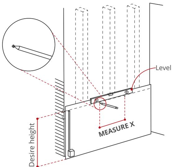
Using a pencil, mark the position of each mounting hole accordingly to the distance you measured of the basin mounting holes. **Make sure the mark position is level.**
