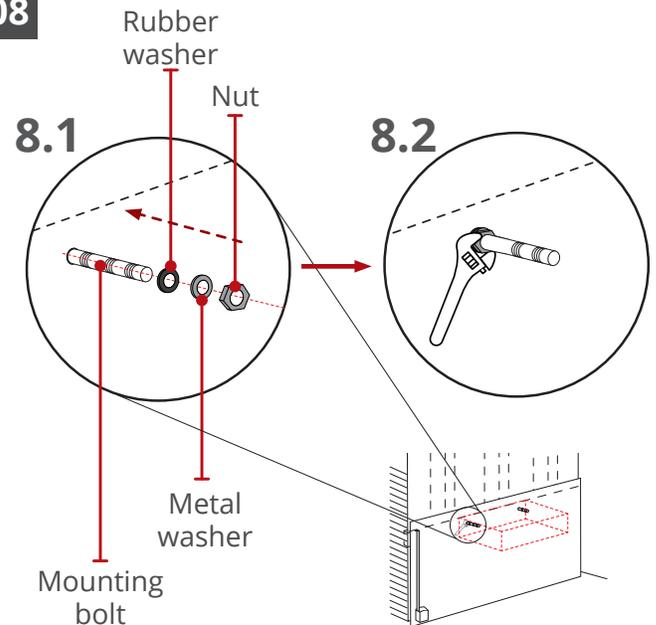
Place rubber washer, metal washer and nuts on to mounting bolts and tighten to secure basin
