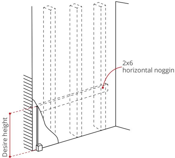
Measure the desire height of the basin and install a 2x6 horizontal noggin.
