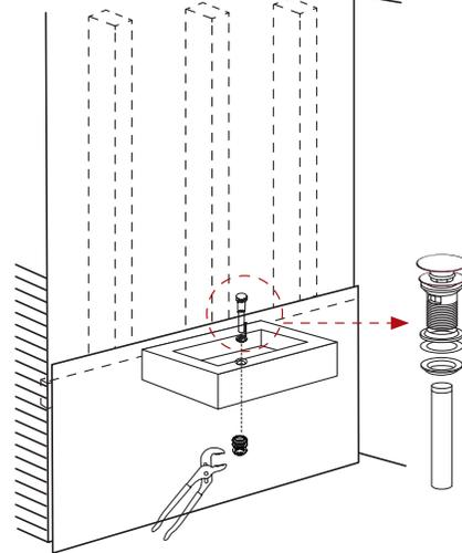
Mount the drain assembly (not included) on the sink following the manufacturer's instructions. Be certain to apply a bead of sealing putty on the underside of the drain in order to ensure a watertight seal between the sink and drain. Remove excess putty after installing drain on sink.
