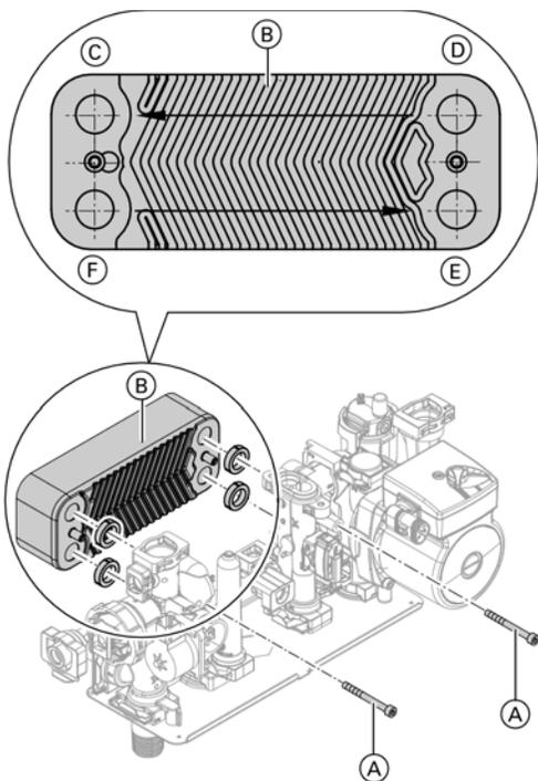
**Checking or replacing the plate type heat exchanger (B1KA only)**
