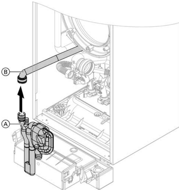
1. Check the siphon to ensure unimpeded drainage of condensate.
