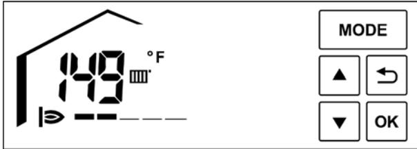
The boiler water temperature reading is constantly displayed during operation.
