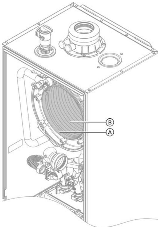
1. Remove burner assembly and reinstall upon completion of service work as per the instructions on page 57 in this manual.
