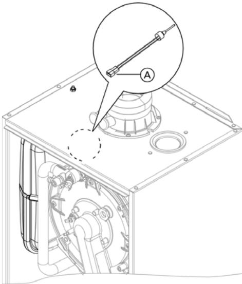
**Check flue gas temperature sensor**
