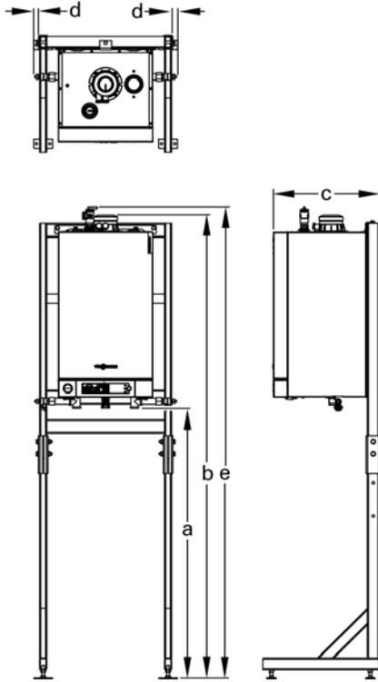
**Boiler mounting frame dimensions**
