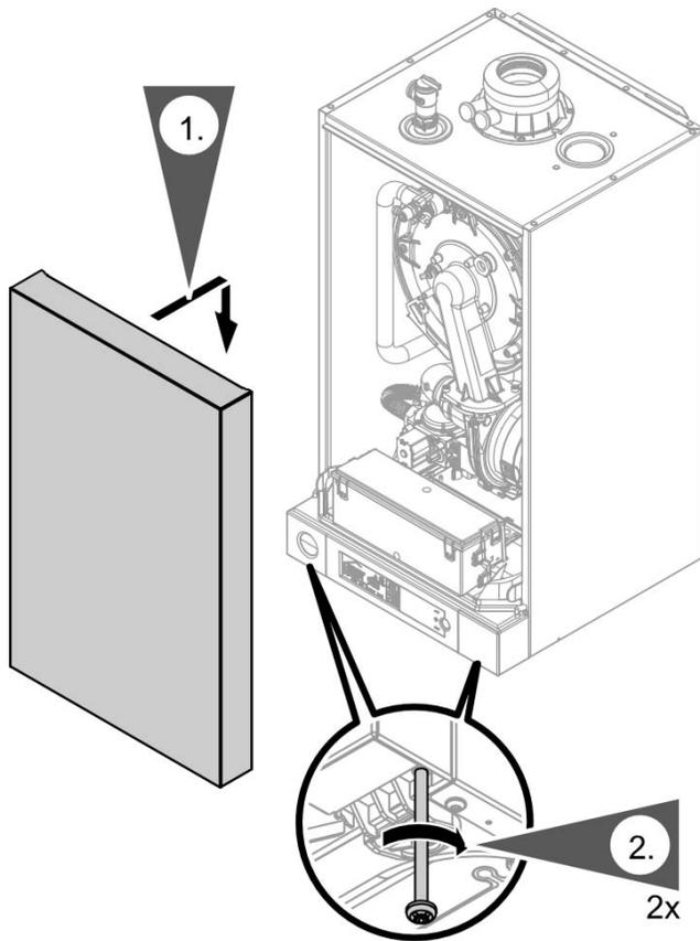
**Reinstalling the front panel**
