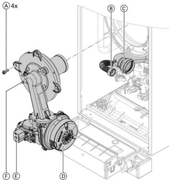
1. Fit burner and tighten 4 T-30 screws (A) diagonally to a torque of 35 lb.in (4 Nm).
