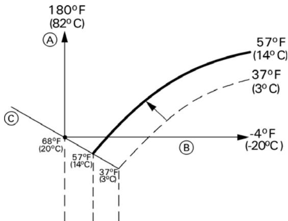
Adjustment of the reduced set point temperature from 37 to 52°F (3 to 14°C)
