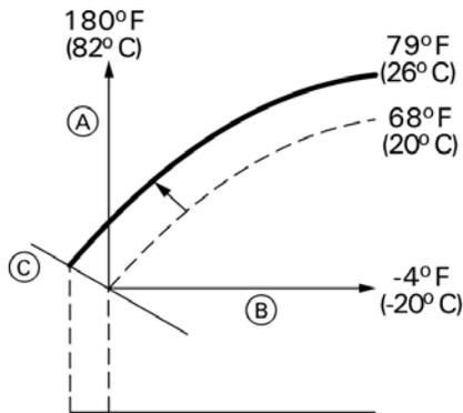
Adjustment of the increase set point temperature from 68 to 79°F (20 to 26°C)
