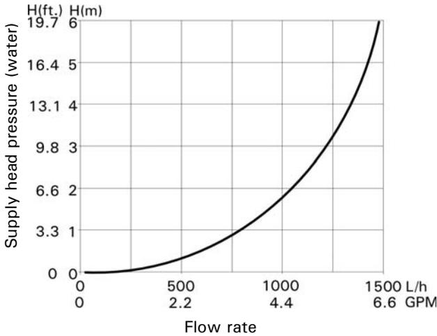
Pressure drop (primary circuit) for Vitodens 100-W, B1HA 26, 35, 94, 125 and B1KA 35, 125 For sizing an on-site circulation system. Max. flow rate: 6.2 GPM (1400 L/h)
