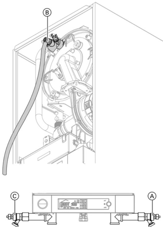
To fill and remove air from the heat exchanger:
