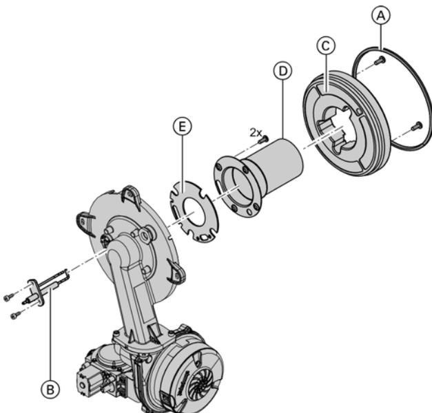
Check the burner gasket (A) and burner cylinder assembly (D) for damage and replace if necessary. Replace the cylinder burner assembly if damaged.
