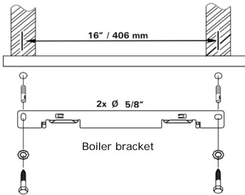
**Boiler mounting bracket installation on metal studs**
