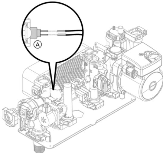
**Check DHW outlet temperature sensor (B1KA only)**
