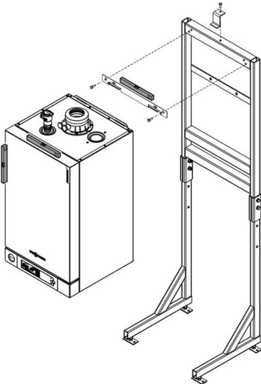
**Boiler mounting bracket and frame**
