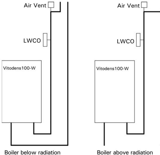
A low water cut-off may be required by local codes. Do not install an isolation valve between boiler and low water cut-off.
