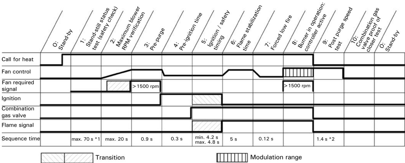
\*1 50 seconds for no flame present check and 20 seconds for blower stand-stil check (total 70 seconds).
