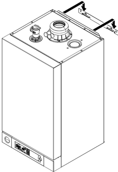
**Mounting the boiler to the wall**
