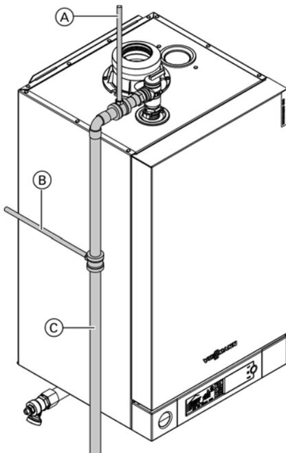
**Installing safety devices on the boiler**
