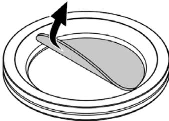
When utilizing the combustion air inlet cover Ⓐ for Vitodens 100-W series boilers, remove the center section and leave the rubber seal in place.
