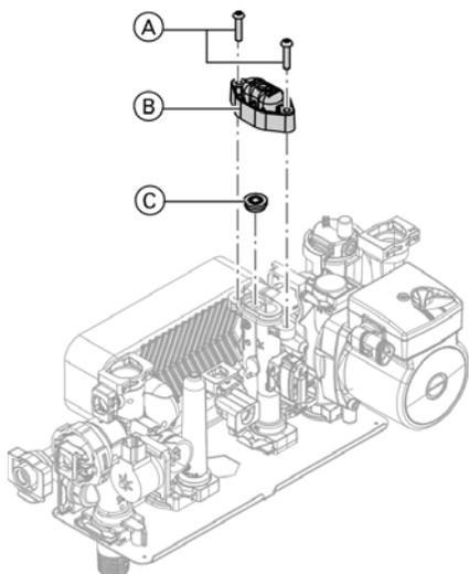
**Replacing the flow limiter (B1KA only)**
