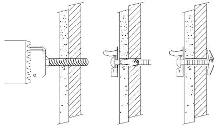
**Boiler Mounting** *(continued)*
