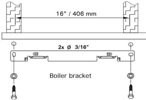
**Boiler mounting bracket installation on wood studs**
