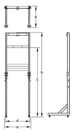
The boiler stand is used for free-standing installation of a single boiler within the mechanical room.
