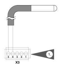
1. Connect the low-loss header sensor (if used) to terminals X3.4/X3.5 on the boiler control board.
