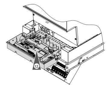
12. Route all connecting cables to the appropriate areas and secure the cables to the control base using existing strain reliefs as shown.
