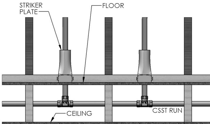
Figure 4.3 Multiple gas outlets connected to the same run of WARDFlex®/WARDFlex®MAX. In this situation a tee-type fitting can be used and installed in a concealed location.
