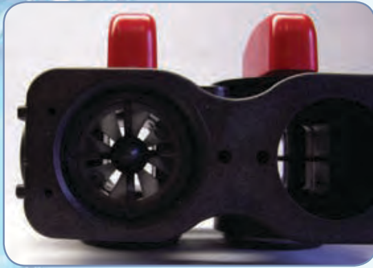
integrated meter in bypass
