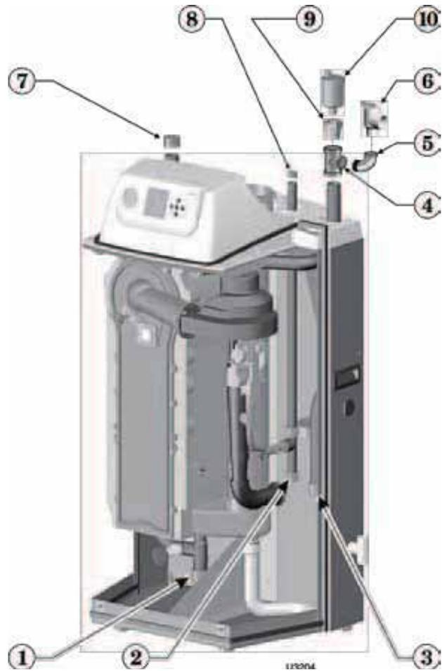
2. Remove pipe caps from bottoms of supply, return and gas lines to route piping through bottom.
