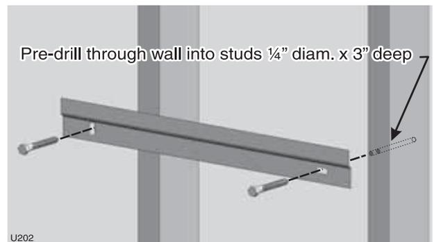
**Figure 46** Place boiler on wall-mount bracket
