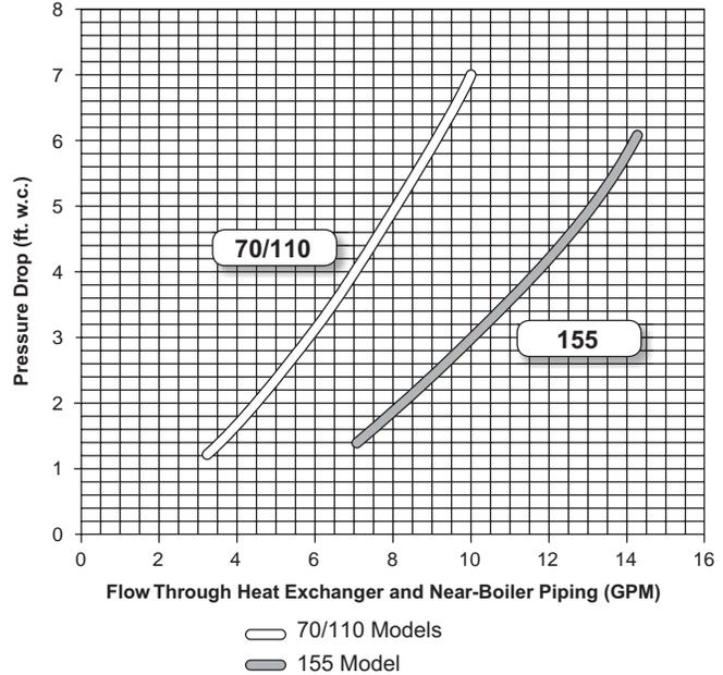
**Figure 51** Estimated head loss of boiler loop piping and recommended circulators.
