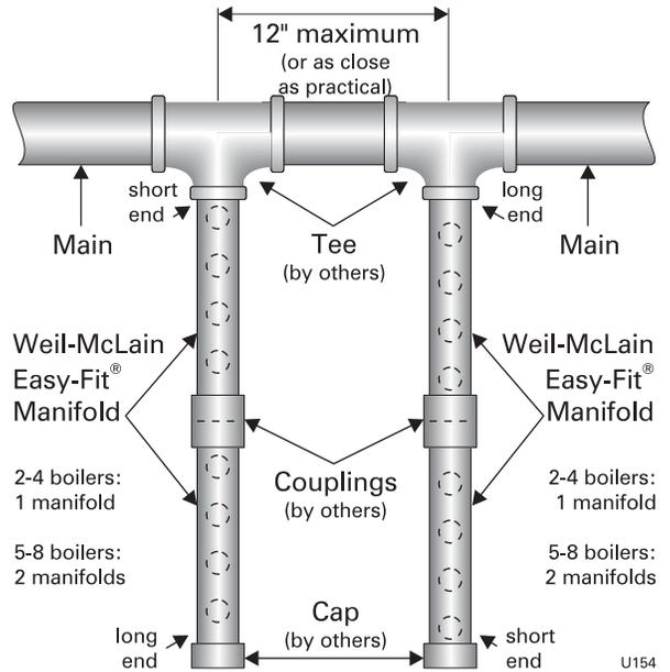
**Figure 59** Double-sided EZ-Fit Header connection
