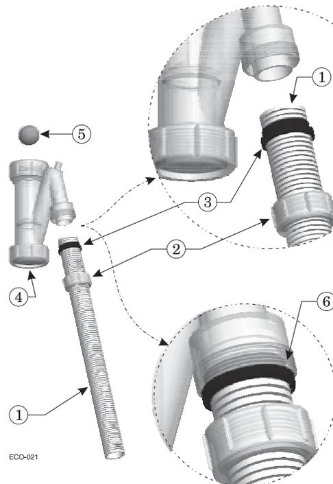
**Figure 63** Condensate trap connection
