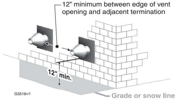
**Figure 31** Installing and supporting the concentric sidewall vent assembly
